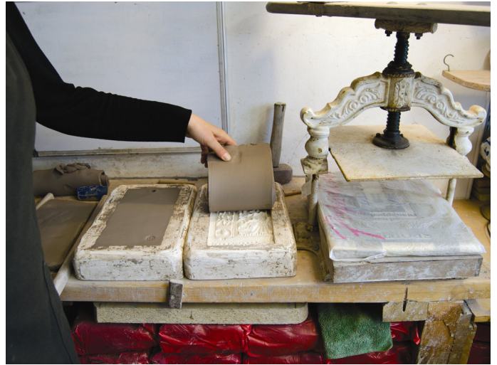
Fig. 5 - Pressing the tiles.
